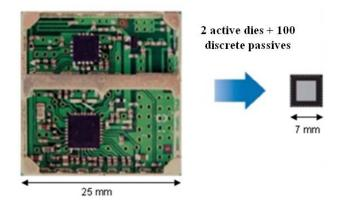
The integration of passive based filters and of decoupling capacitors allows a reduction in size by a factor of yy, meaning a space saving of more than 80 mm2. It is also very obvious that in such an integration approach, the replacement of around 100 discrete components by a single Silicon chip will reduce significantly the number of interconnections, hence improving the reliability of the final product.
