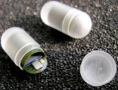
This device is an electronic pill including a sensor, a secured wireless communication module and of course its source of energy. It is only measuring 15mm long and 6mm in diameter. Making possible the realization of this product has been made with the use of Integrated Passives. In this product, the 5x6 mm PICS die is incorporating more than 150 passive components. Without these technologies, such a device could not be made.
