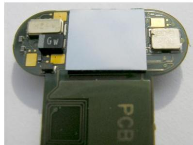
*Figure 5: Example of SiP-WLCSP: a controller, RF communication and sensor die set is flipped over a PICS interposer in WLCSP package architecture, and the flex application in medical domain*
