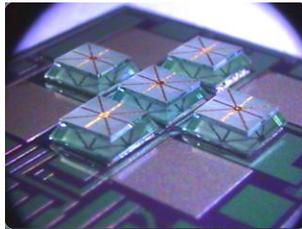
*Figure 4 : Example of PICS interposer in LED application : 4 LEDs are flipped over PICS and 5 LEDs are stacked above PICS*
