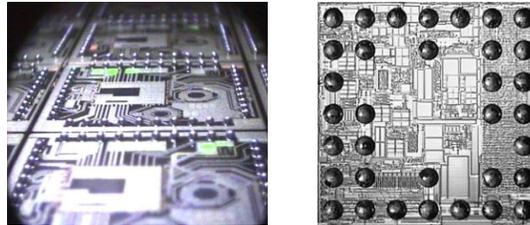
*Figure 2: Examples of PICS in WLCSP package architecture*
