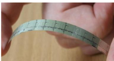
*Figure 1: Sample of IPD using the  $250\text{nF}/\text{mm}^2$  technology thinned at  $60\mu\text{m}$ .*
