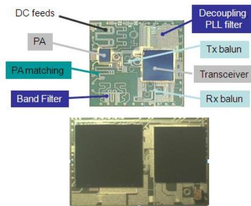
Figure 3: Examples of PICS interposer in RF application (top) and Digital TV with channel decoder, Silicon tuner and LNA transistor functional die (Bottom)
