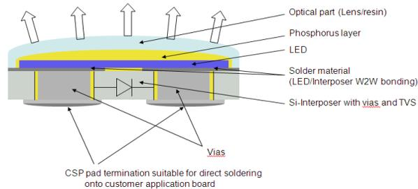
Figure 6 :Example of PICS interposer with via used in W2W technology for LED domain
