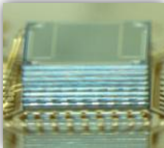
Fig.8: a 33µF Capacitor in a package size of 4.8mm*4.4mm*2 mm
