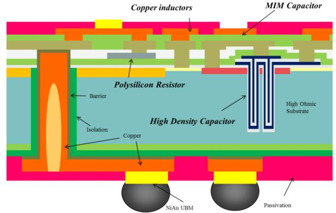
Figure 5: Silicon interposer with TSVs and High Density Capacitors, Polysilicon Resistors, MIM capacitor and Copper inductors .
