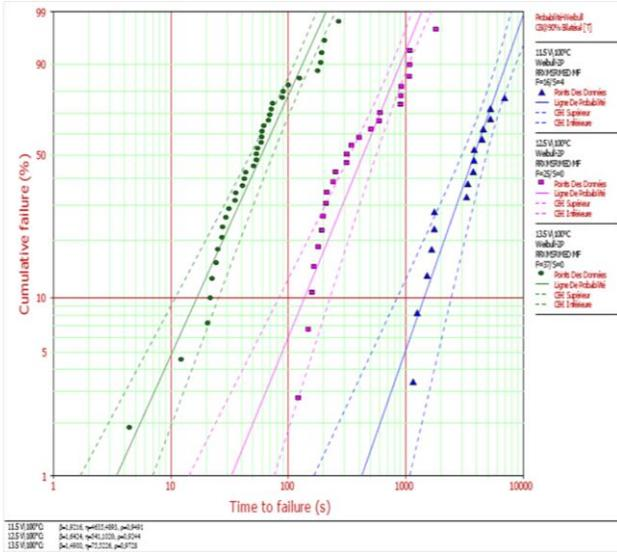
Figure 4: TTF when dielectric is exposed to 3 voltages : 11.5V, 12.5V, 13.5V
