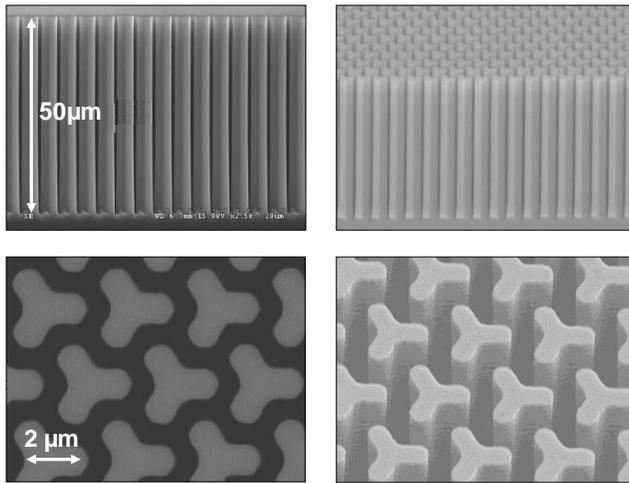
Figure 1: SEM pictures of the high aspect-ratio pillars etched in the silicon substrate (tripods of AR= 50:1)
