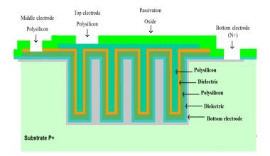
Figure 2: cross sectional view of the MIMIM architecture.
