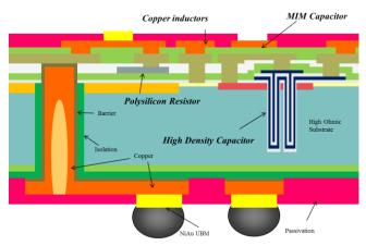
Figure 5: Silicon interposer with TSVs and High Density Capacitors, Polysilicon Resistors, MIM capacitor and Copper inductors .
