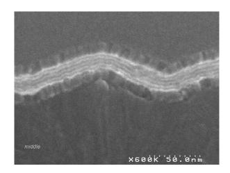
Figure 3: higher k-dielectric nanolaminates deposited in high aspect ratio 3D structures.
