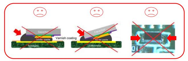
Figure 2: Solder paste after reflow - Rejected
