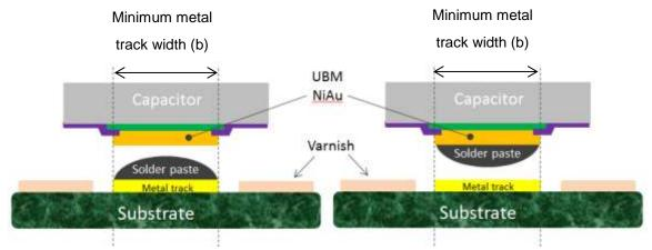
Figure 1.3: unbumped capacitor
