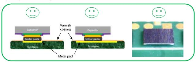
Figure 1: Solder paste after reflow - Targeted
