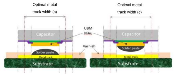
Figure 1.5: unbumped capacitor
