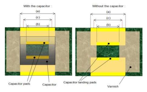
Figure 1.7: design of the substrate
