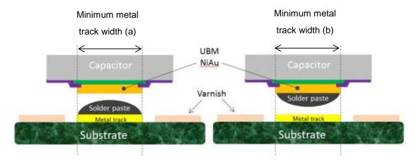
Figure 1.1: unbumped capacitor
