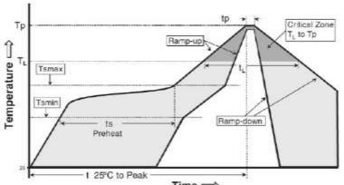
Figure 3: Generic reflow profile according to JEDEC J-STD-020-C
