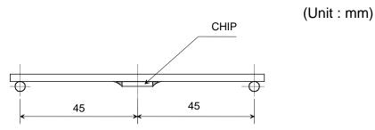
Test method (Unit : mm)
