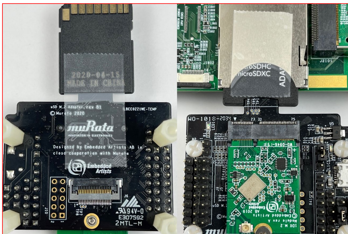
Figure 30: Securing uSD/SD Connection on i.MX 6 EVK
