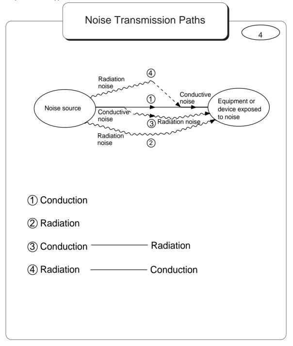
Noise emitted from a source is transmitted through many complicated paths, sometimes through a conductor and sometimes as radiation. When it reaches a device or equipment, that equipment is exposed to noise.
