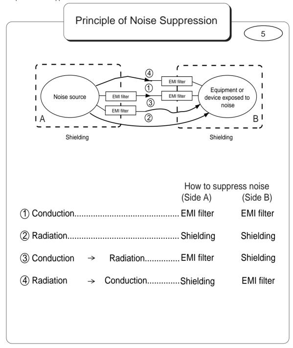
In order to properly suppress noise, we must know the noise source and how it is transmitted. If the initial check is inaccurate, we cannot judge whether the noise suppression technique has failed or the technique was applied to an incorrect source.
