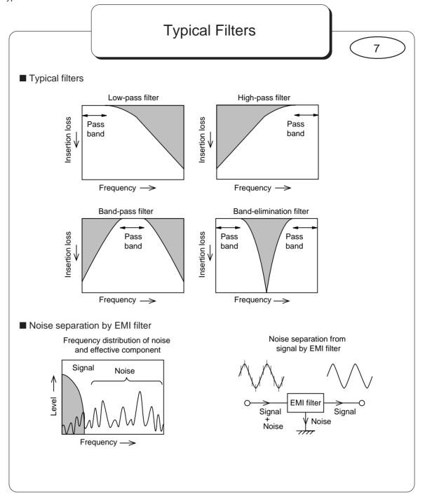
Filters used to pick out the desired signals are classified into the following four types.
