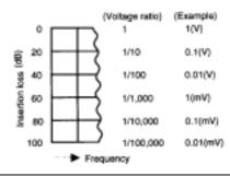
The noise suppression performance of EMI filters is measured according to the measuring method of insertion loss specified in MIL STD-220. Voltage across a load is measured both with and the expression shown above. The unit of insertion loss is expressed in dB (decibel). For example, when insertion loss is 20 dB, noise voltage is reduced to one-tenth.
