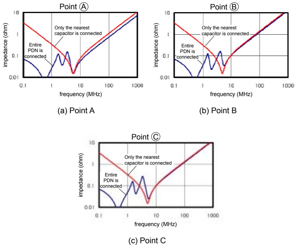
Figure 7-2 Calculation results of power supply impedance
