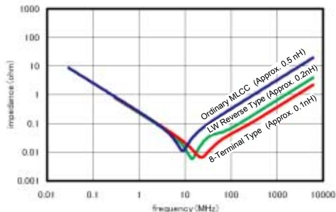
Figure 4-5 An example of impedance characteristics for a low-ESL capacitor
