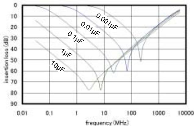
Figure 2-8 Insertion loss characteristics of capacitor (Converted from Data in Murata Chip S-Parameter & Impedance Library)
