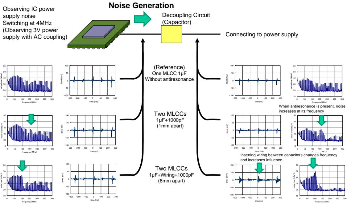
Figure 3-15 Examples of noise observation when antiresonance is present
