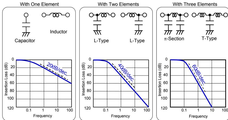
Figure 5-11 Insertion loss characteristics of LC filters
