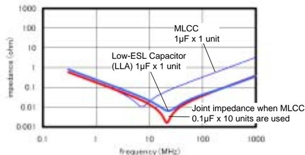
Figure 8-13 Comparison between using MLCCs in parallel and a low-ESL capacitor (calculated values)
