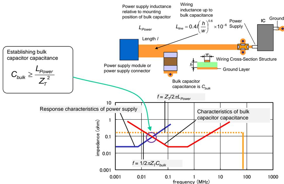
Figure 8-16 Establishing capacitance for a bulk capacitor
