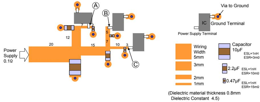
Figure 7-1 Modeling diagram of power supply impedance calculation
