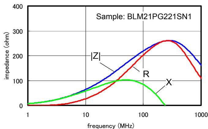
Figure 5-8 Frequency characteristics for ferrite bead impedance
