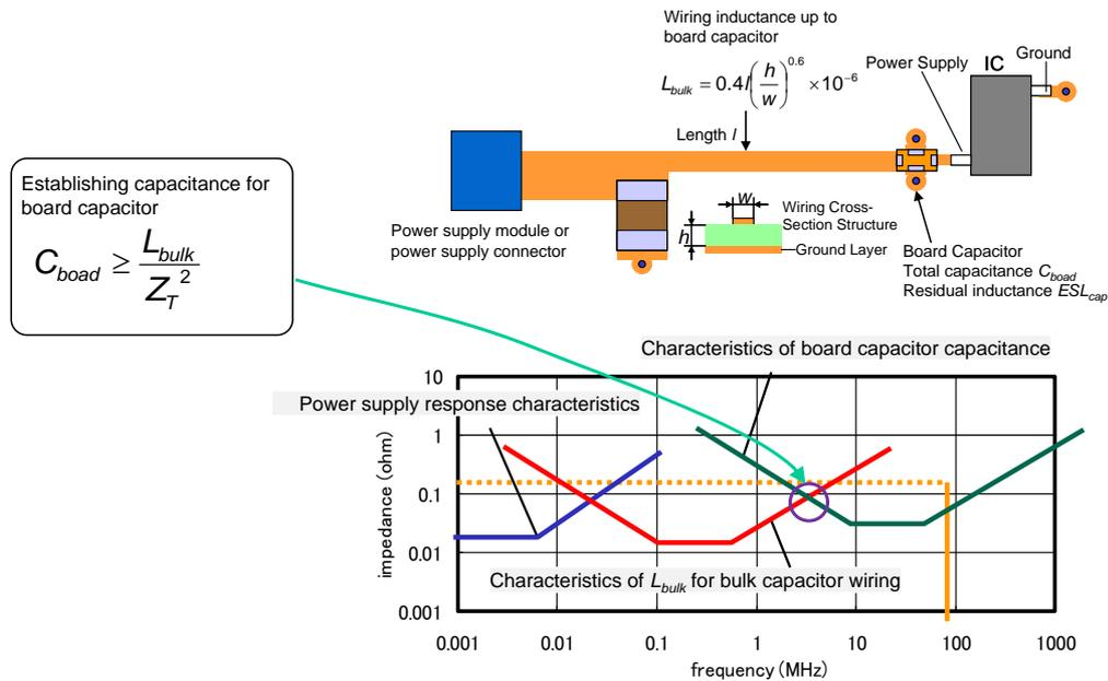
Figure 8-17 Establishing board capacitor capacitance
