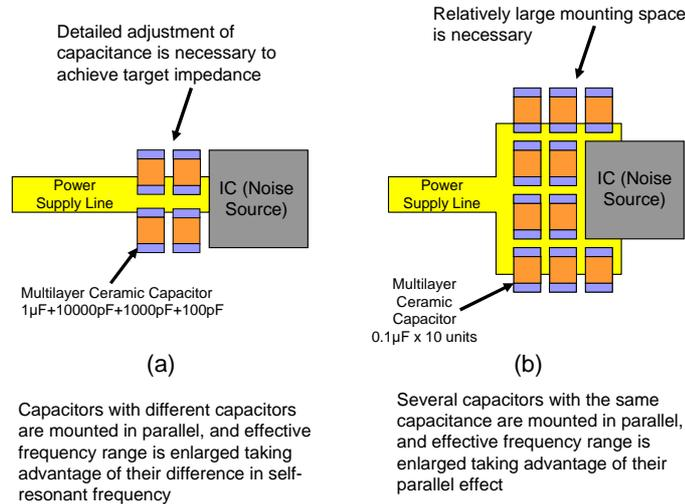
Figure 8-10 Examples of board capacitor parallel layout
