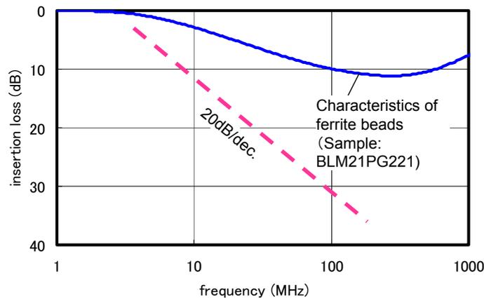
Figure 5-9 An example of insertion loss characteristics for a ferrite bead
