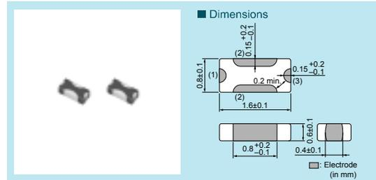
High capacitance type up to 2.2 $\mu$ F NFM18PC series
