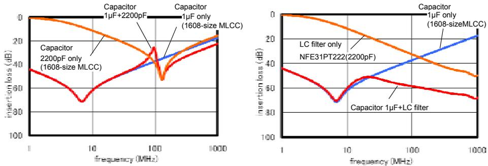
(a) When combining two capacitors (b) When combining a capacitor and a LC filter
