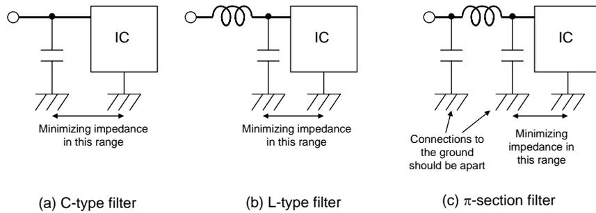
Figure 2-9 Filter configurations used for IC power supplies
