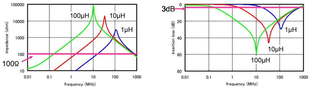
Figure 5-4 Comparison of impedances and insertion losses of inductors
