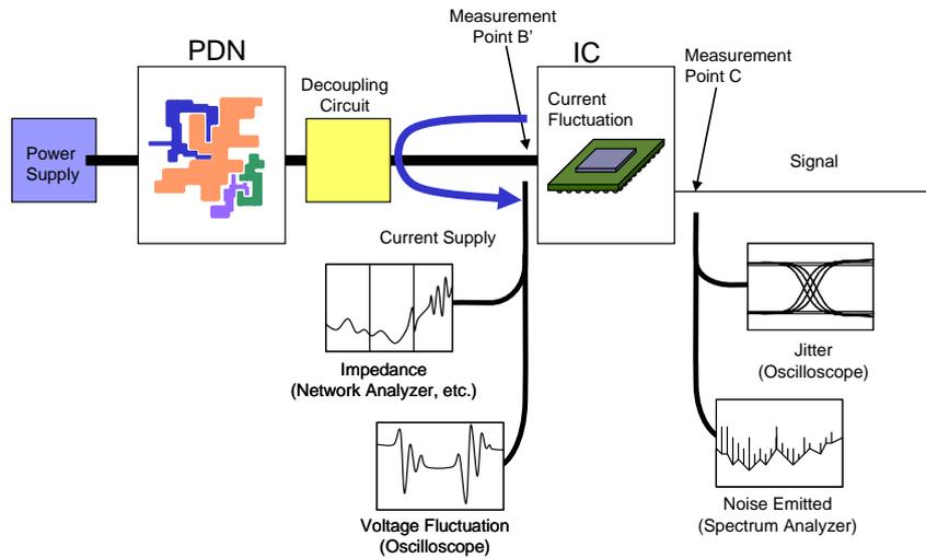
Figure 2-4 Measurement to evaluate current supply performance
