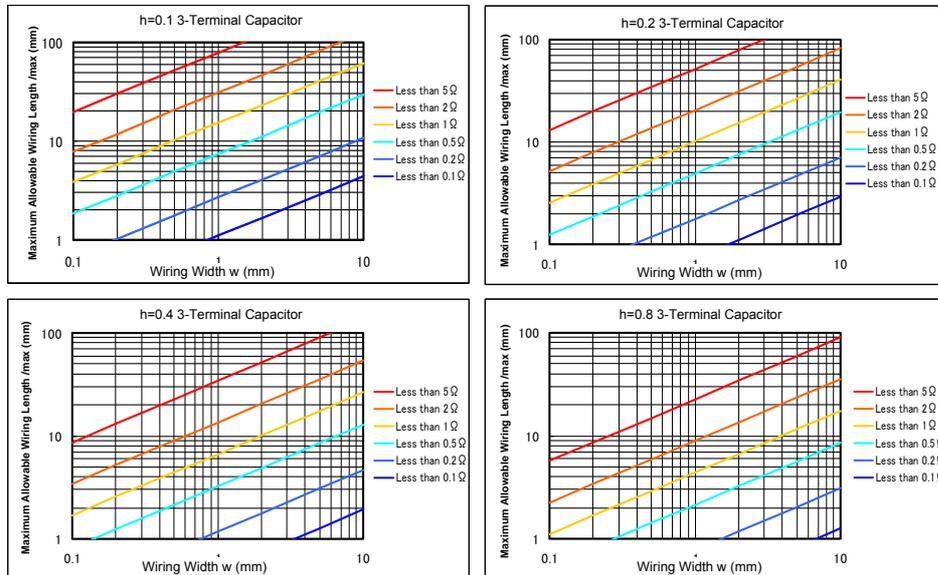
Figure 7-7 3-Terminal Capacitor Best Conditions ( $ESL_{cap}=0.05nH$ )
