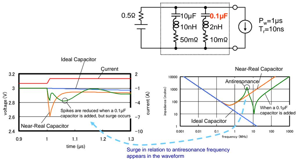
Figure 6-9 When parallel capacitors are resonating
