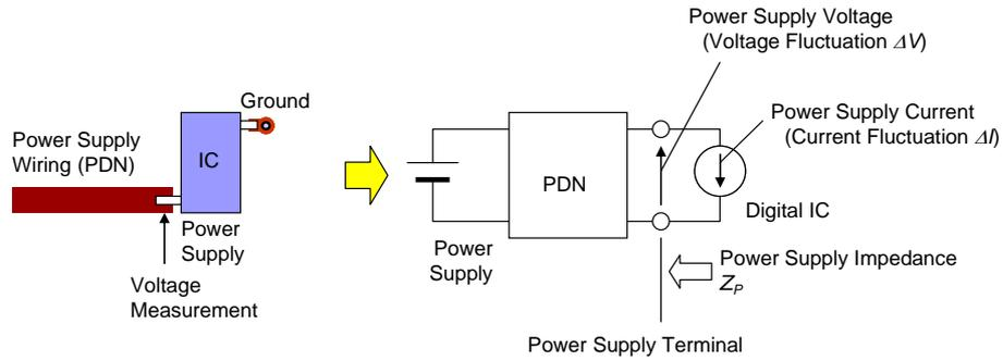
Figure 6-2 Measurement position of voltage fluctuation
