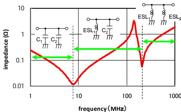
Figure 3-13 Mechanism of the capacitor's parallel resonance
