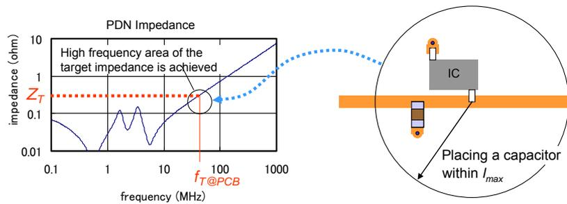
Figure 7-4 Placing a capacitor within  $l_{max}$
