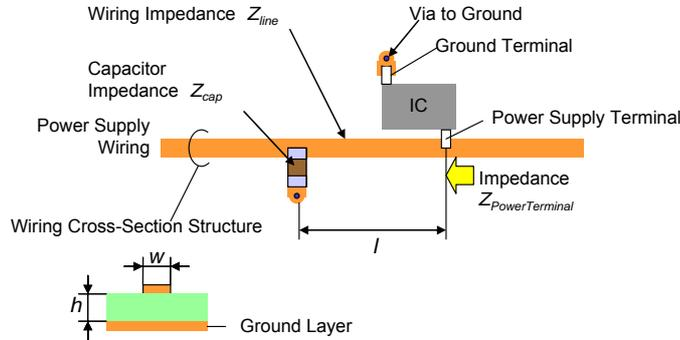
Figure 7-3 Wiring model to the nearest capacitor
