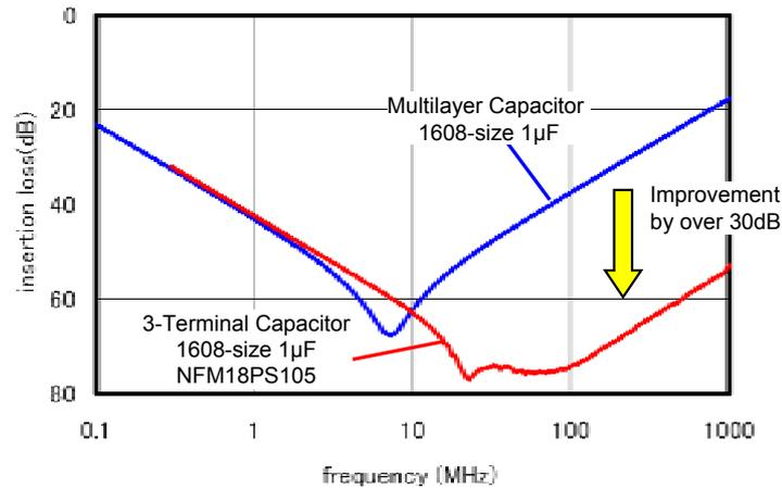
Figure 4-9 Insertion loss characteristics of a 3-terminal capacitor
