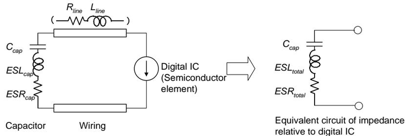
Figure 8-5 Equivalent circuit for a single capacitor
