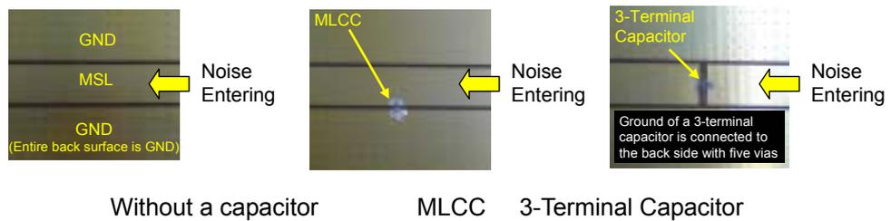
(C) Reference: Mounted state of a capacitor (wiring thickness is for (b)  $3\Omega$ )
