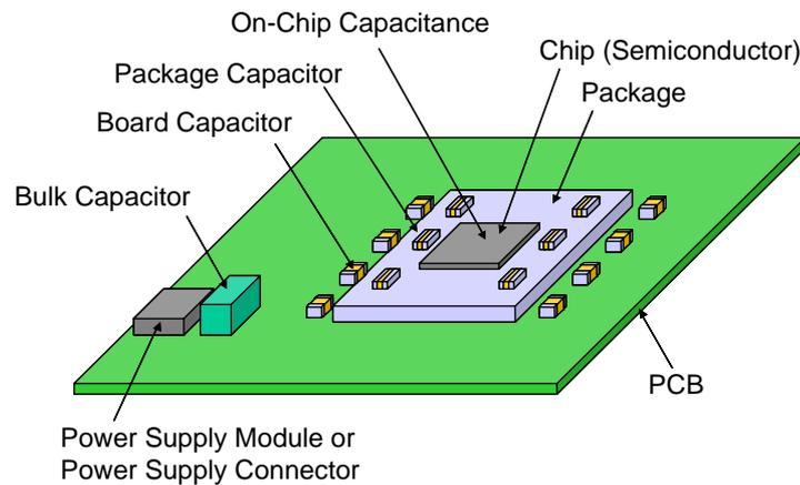
Figure 8-1 An example of decoupling capacitor placement
