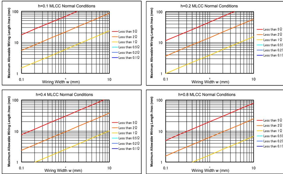
Figure 7-10 MLCC Normal Conditions ( $ESL_{cap}=1nH$ )
