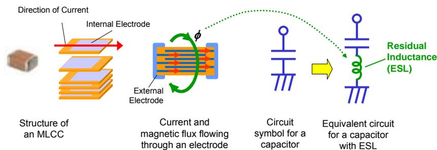
Figure 4-1 Mechanism of ESL generation in an MLCC
