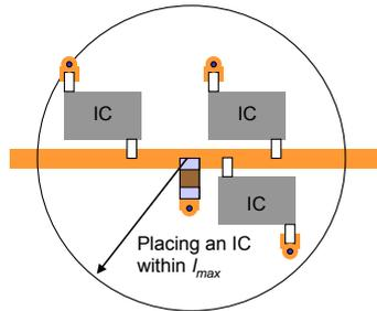
Figure 7-5 Placing an IC within  $l_{max}$
