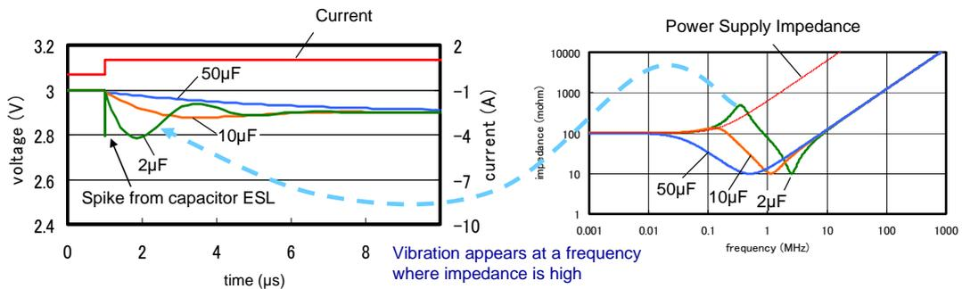
Figure 6-12 Calculation results when pulse width is wide
