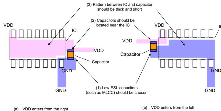
Figure 2-2 An example of decoupling capacitor positioning
