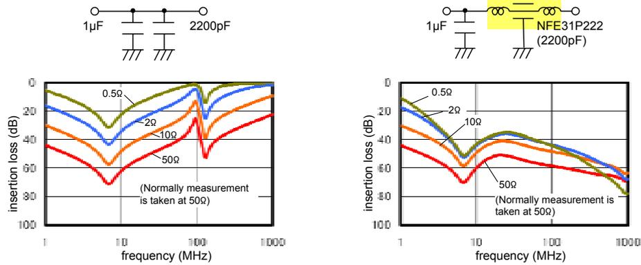
(a) When combining two capacitors      (b) When combining a capacitor and an LC filter
