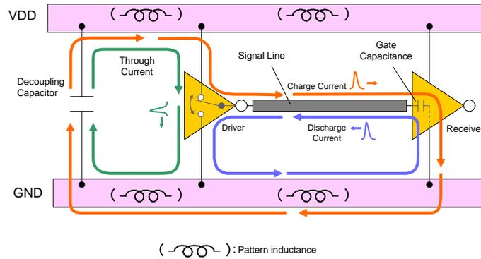
Figure 2-1 Simplified model of a digital IC
