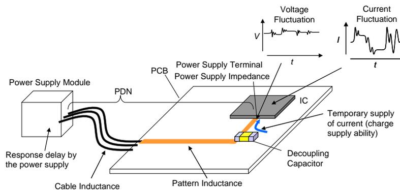
Figure 6-1 Current and voltage fluctuations
