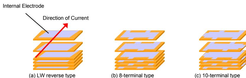
Figure 4-3 Structure of low-ESL capacitor (schematic view)
