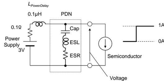
Figure 6-11 Simulation circuit when pulse width is wide
