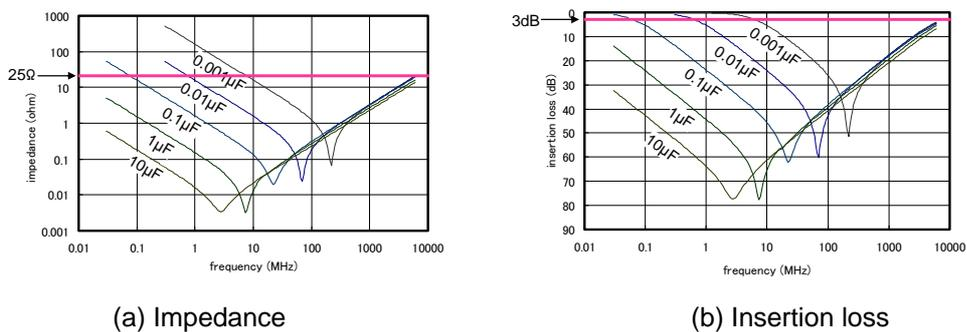
(a) Impedance (b) Insertion loss
