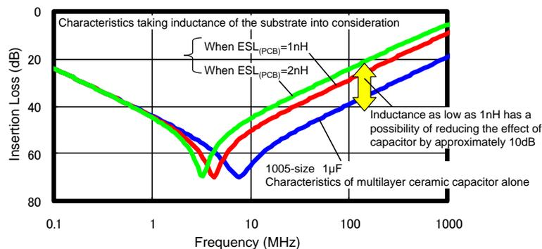
Figure 3-5 Fluctuation in characteristics of conductor due to mounting inductance (calculated values)
