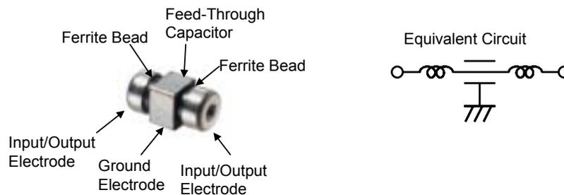
Figure 5-15 LC filter NFE31 for power supplies
