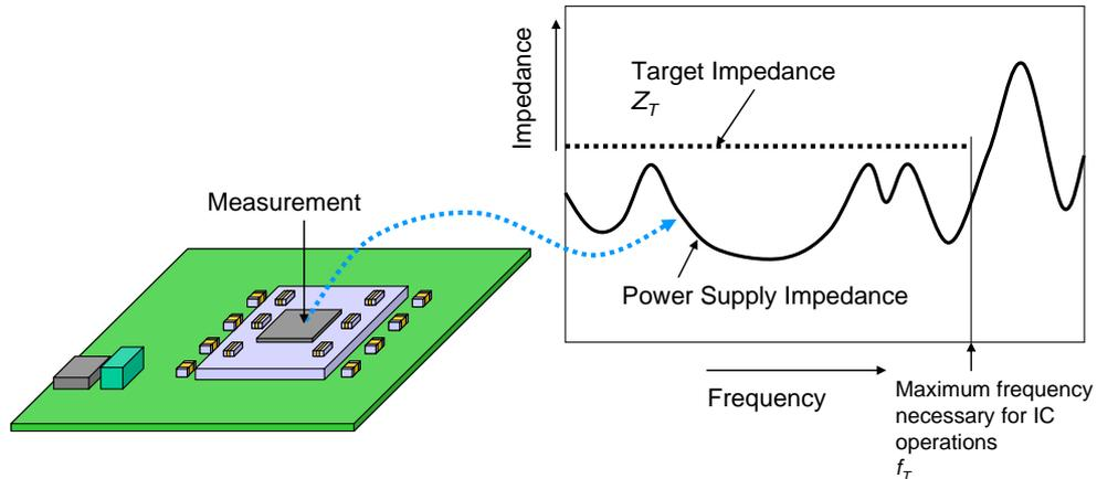
Figure 8-3 Target impedance
