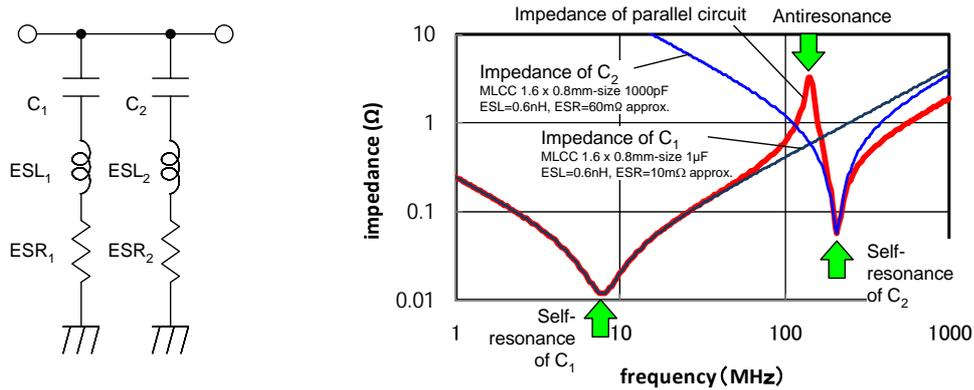
Figure 3-12 Parallel resonance of the capacitor (calculated values)
