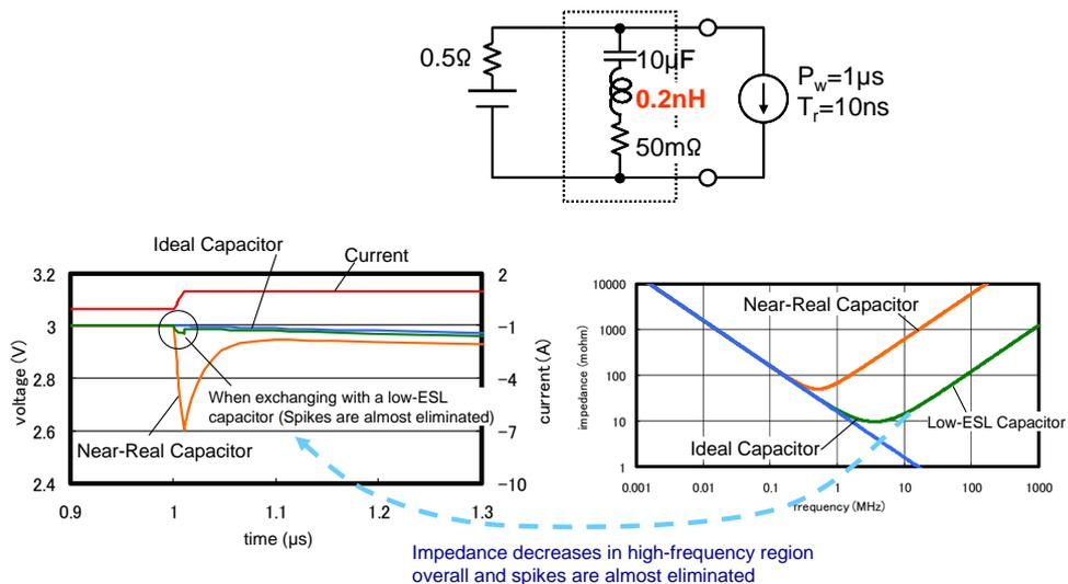
Figure 6-10 When using a capacitor with small ESL
