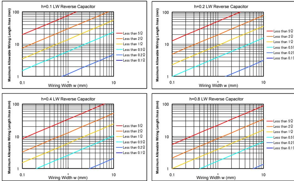
Figure 7-8 LW Reverse Capacitor Best Conditions ( $ESL_{cap}=0.2nH$ )
