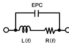
Figure 5-7 Equivalent circuit for a ferrite bead
