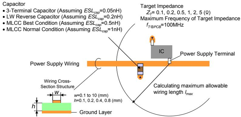
Figure 7-6 Calculation conditions
