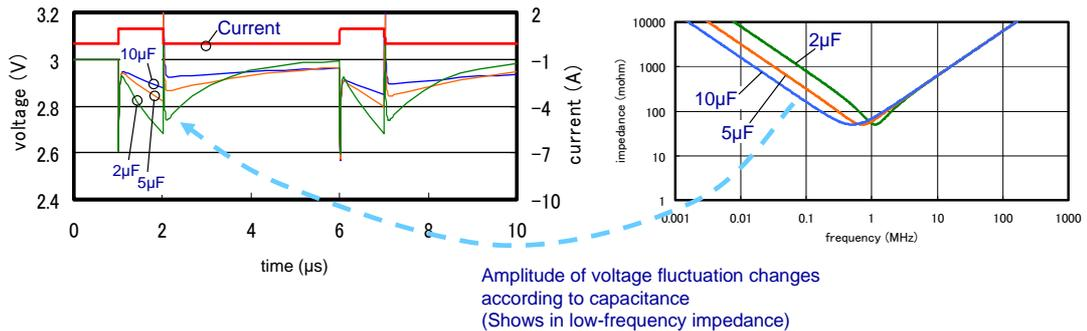
Amplitude of voltage fluctuation changes according to capacitance (Shows in low-frequency impedance)
