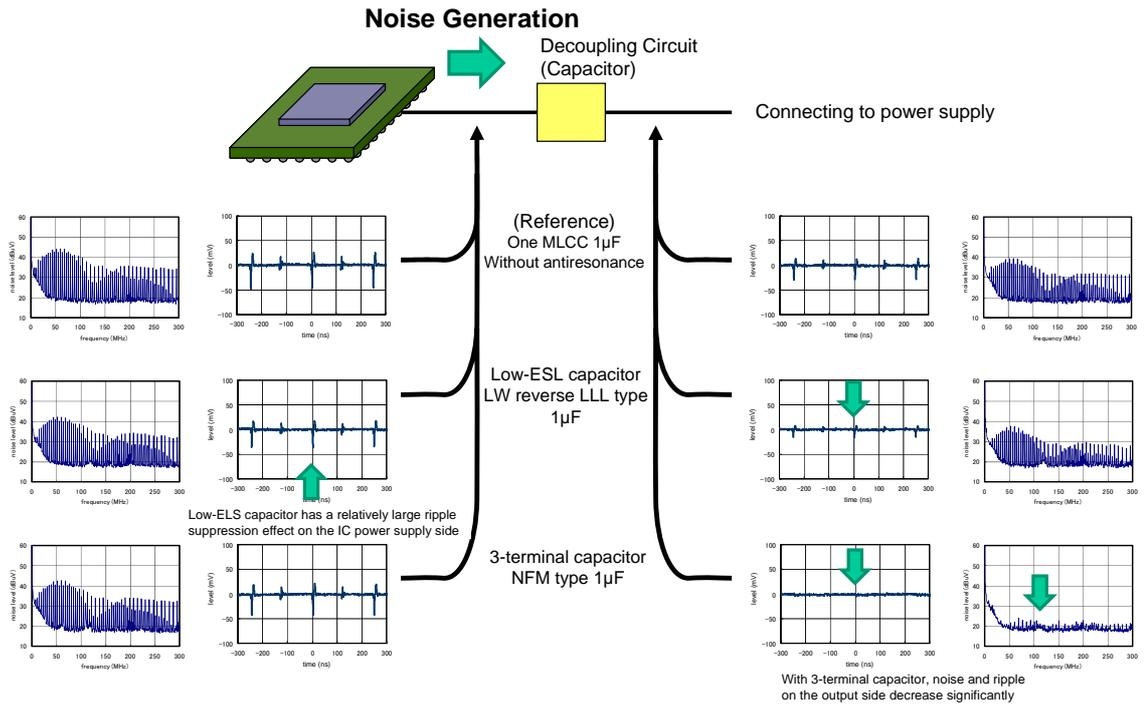
Figure 3-17 Measurement results when using low-ESL capacitors
