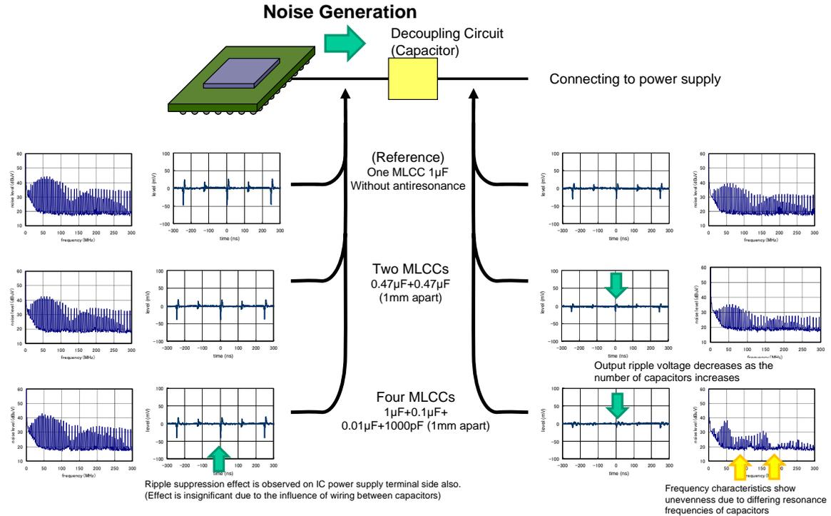
Figure 3-16 Measurement results for combinations with little antiresonance
