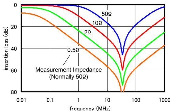
Figure 5-5 Fluctuation in insertion loss in relation with measurement system impedance
