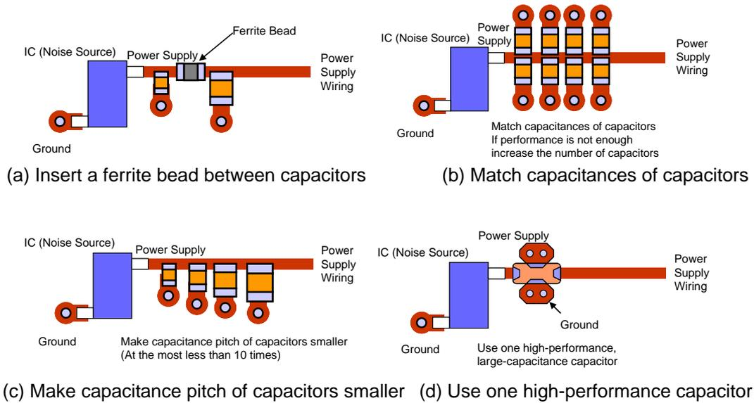
Figure 3-14 Examples of positioning capacitors to suppress antiresonance
