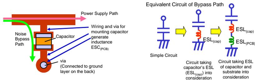
Figure 3-4 Influence of wiring when mounting a capacitor
