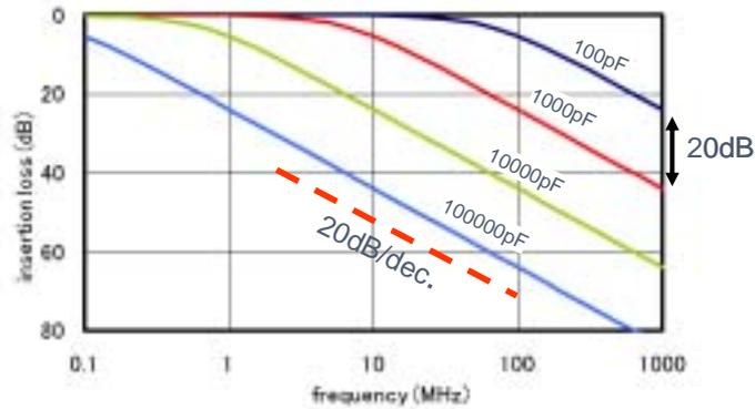
Figure 2-7 Insertion loss characteristics of capacitor (theoretical values)
