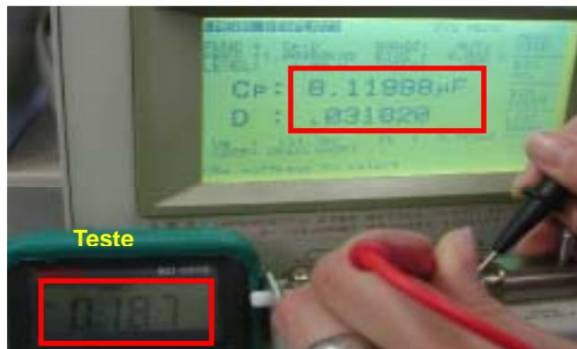
Fig.21 Tester Measurement Example for ALC OFF State
