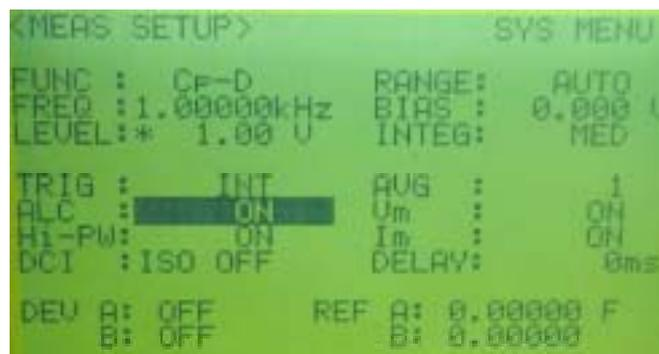
Fig.13 Measure Setup Screen
