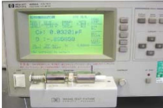
Fig.24 Meter with Measuring Jig installed on
