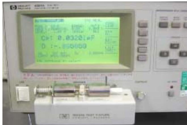
Fig.12 LCR Meter with Jig Installed
