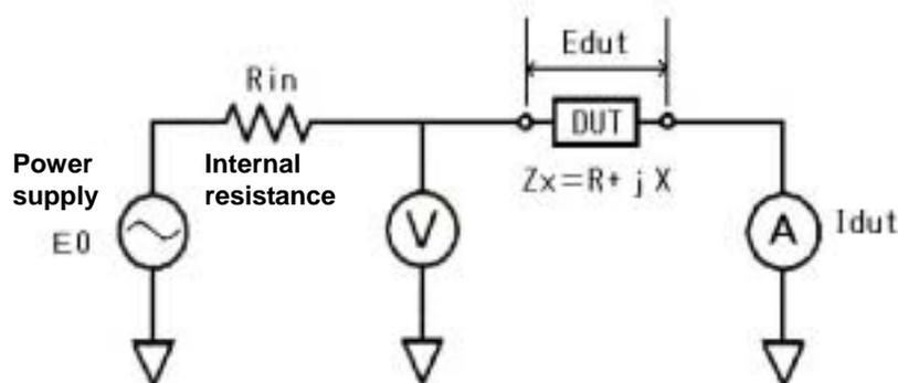
Fig.8 Measuring Voltage Applied to DUT
