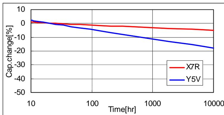
Fig. 27 Aging Characteristic, Capacitance Change with Time
