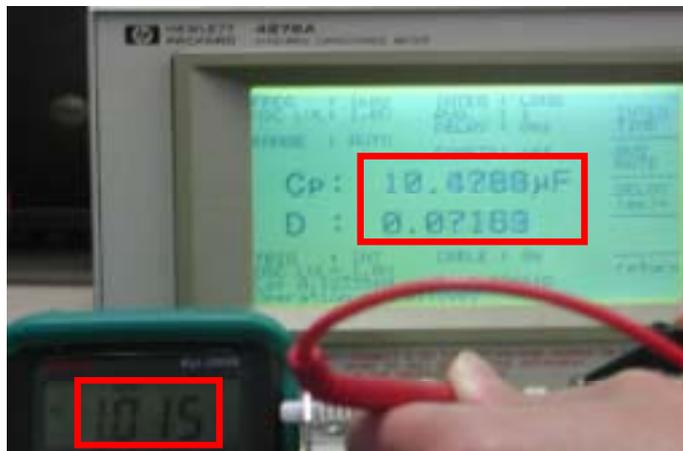
Fig.26 Measurement Voltage Check by Tester
