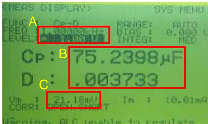
"A" field in the above figure is set to "FREQ: 1kHz" and "LEVEL: 1V", both of which are different from sample's specification. The capacitance indicated in "B" field above is very low, about 75μF against nominal value of 100μF of the sample capacitor, which is 20% lower than that measured by the correct conditions. "Vm" in "C" field indicates the actual measurement voltage monitored by the meter, which shows only about 21mv against set value 1V.
