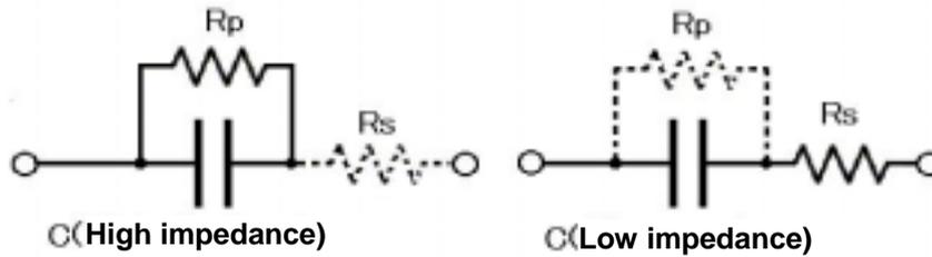
Fig.9 Small capacitance
