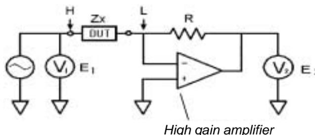
Fig.7 Principle Diagram of Automatic Balancing Bridge
