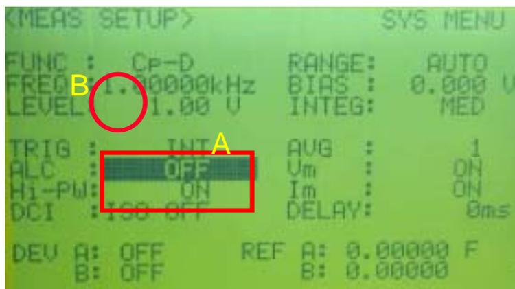
"A" field in the above figure indicates ALC being set to "OFF" and Hi-PW being set to "ON". No asterisk mark at "B" field in the figure means ALC is off.
