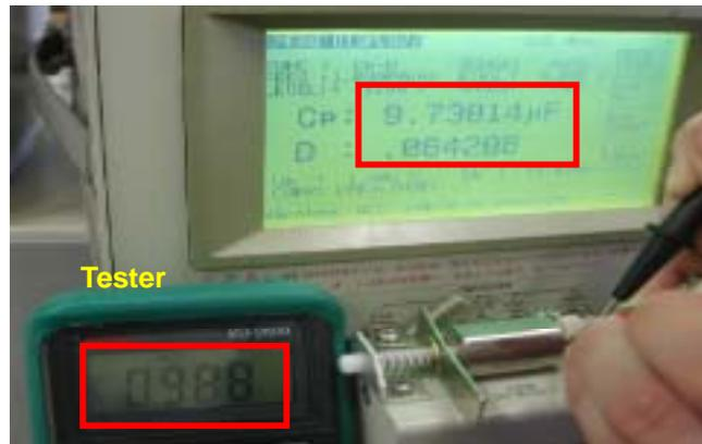
Fig.20 Tester Measurement Example for ALC ON State
