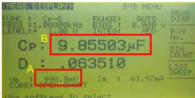
"Vm" in "A" field in the above figure indicates actual measurement voltage monitored by the meter, which shows 1V being applied to the sample. "B" field shows the capacitance of a 10μF product, which is about 9.86μF which is within the specified tolerance.
