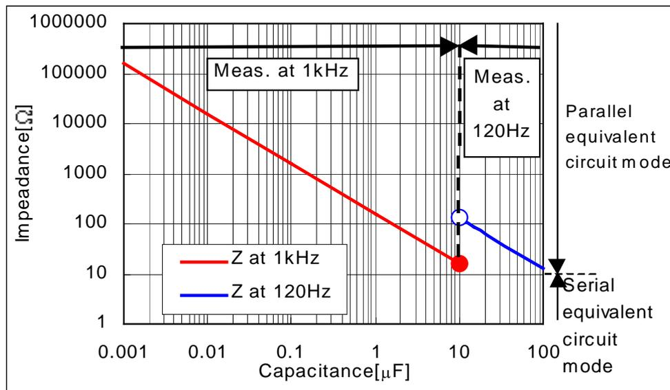
Fig.11 Relation between Capacitance and Impedance
