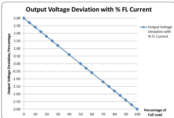
No external current signal bus connection is required (as with active current sharing) which provides a robust method of sharing. As the power supplies might not share within defined tolerances during ramp up phase, it is recommended to limit the load to the capability of a single power supply during startup.
