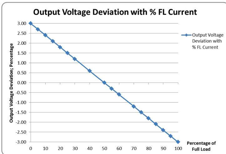
The system load will demand a specific current and each power supply “positions” itself appropriately on the droop curve.
