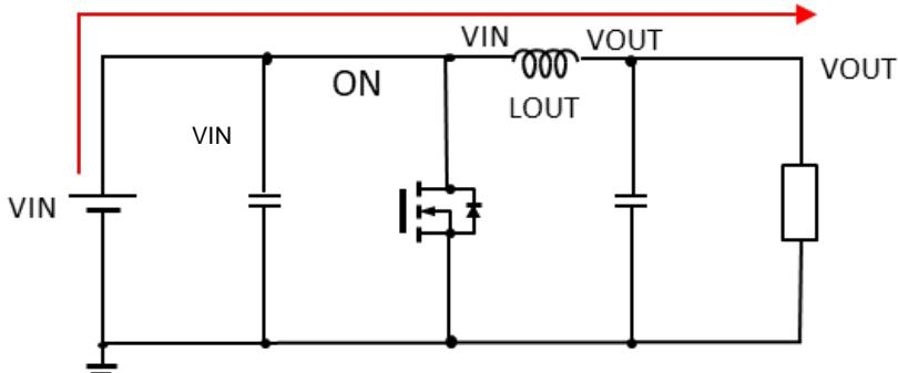
Figure 4. Step-down converter (State 1: High side FET ON)
