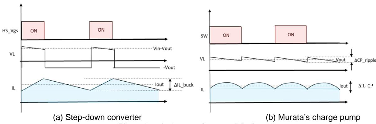
Figure 5. Inductor voltage and ripple current
