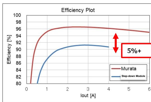
Figure 7. Efficiency characteristics (VIN=48V, VOUT=12V)
