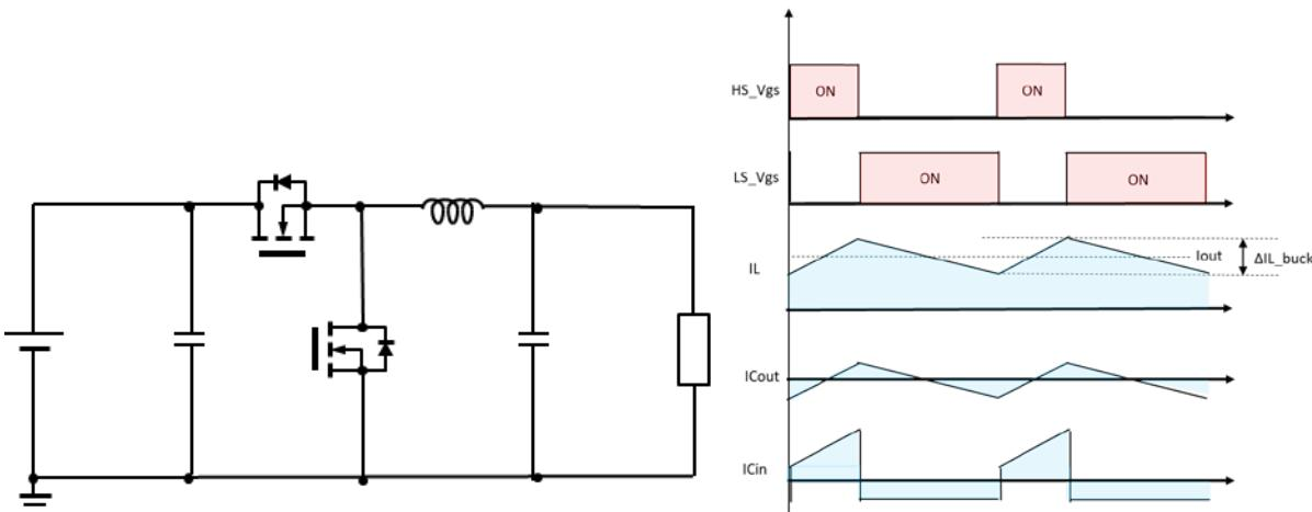
Figure 2. Step-down converter
