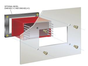
Four ABS-plastic bezel assemblies are available (see Ordering Guides) for aesthetics or environmentally-demanding applications. For those applications requiring moisture and/or dust resistance, two bezels are offered with EPDM sealing gaskets. The gasket is installed around the meter and seals the perimeter of the bezel/meter/panel interface. For added durability, all bezels feature threaded metallic screws and inserts.
