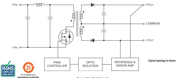
Figure 1. Simplified Schematic
