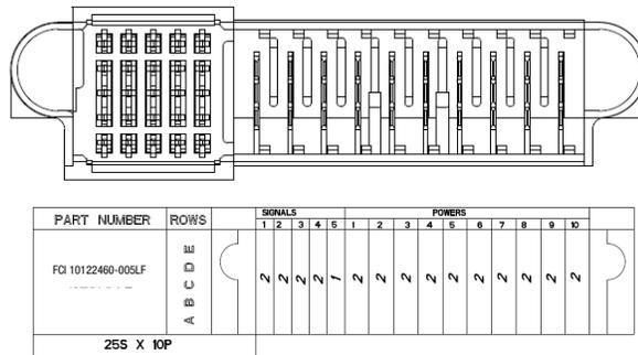
Note: "2" refers to the longest signal pin/power blade & "1" is the "shortest" signal pin such that the "shortest" is the "last to make, first to break" in the mating sequence.
