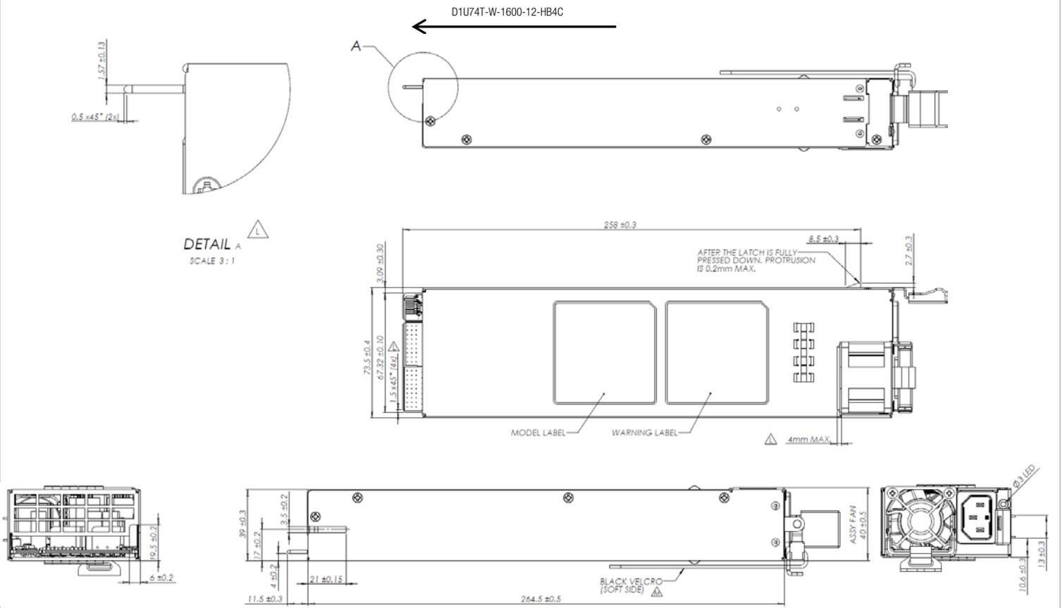
1. AC input connector: IEC 60320-C14
