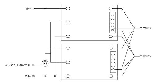
Figure 3. Load Sharing Block Diagram
