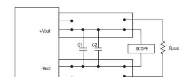
$C1 = 1\mu F; C2 = 10\mu F$ LOAD 2-3 INCHES (51-76mm) FROM MODULE
