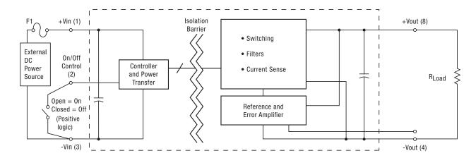
Figure 1. Connection Diagram (without digital interface)
