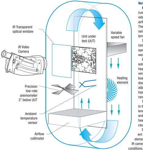
Figure 8. Vertical Wind Tunnel
