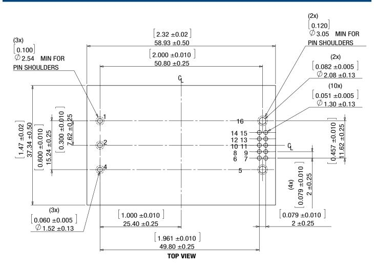
600W Digital Fully Regulated Intermediate DC-DC Bus Converter
