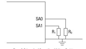
Figure 2. Schematic of Connection of Address Resistors
