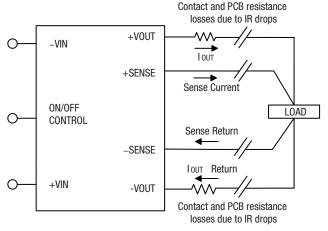
Figure 6. Remote Sense Circuit Configuration
