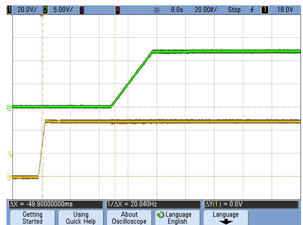
Figure 12. Vin Start-up Delay (CH2: Vout, CH1: Vin) (Vin=48V, Iout=50A, Cload=330μF, Ta=+25°C, 20mS/div)
