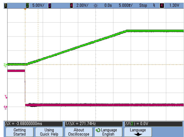
Figure 12. Vin Start-up Delay (CH2: Vout, CH1: Vin) (Vin=48V, Iout=50A, Cload=330μF, Ta=+25°C, 20mS/div)
