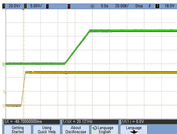
Figure 11. Vin Start-up Delay (CH2: Vout, CH1: Vin) (Vin=48V, Iout=0A, Cload=330μF, Ta=+25°C, 20mS/div)
