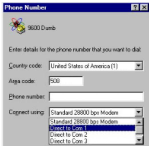
Figure 8. Direct to Com Port Setting
