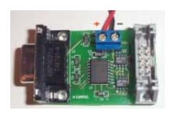
Figure 4. DTL-RS232-485 Adapter Card
