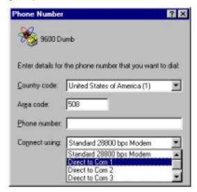
Figure 8. Direct to Com Port Setting
