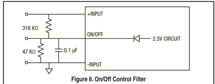
Figure 6. On/Off Control Filter
