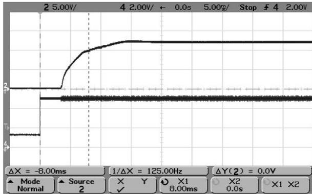
**Power On Startup Delay Output**
