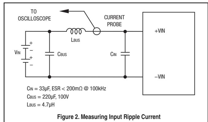
In critical applications, output ripple and noise (also referred to as periodic and random deviations or PARD) may be reduced by adding filter elements such as multiple external capacitors. Be sure to calculate component temperature rise from reflected AC current dissipated inside capacitor ESR.
