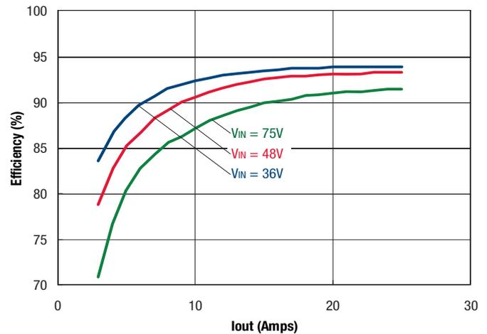
Efficiency vs. Output Current @ +60°C
