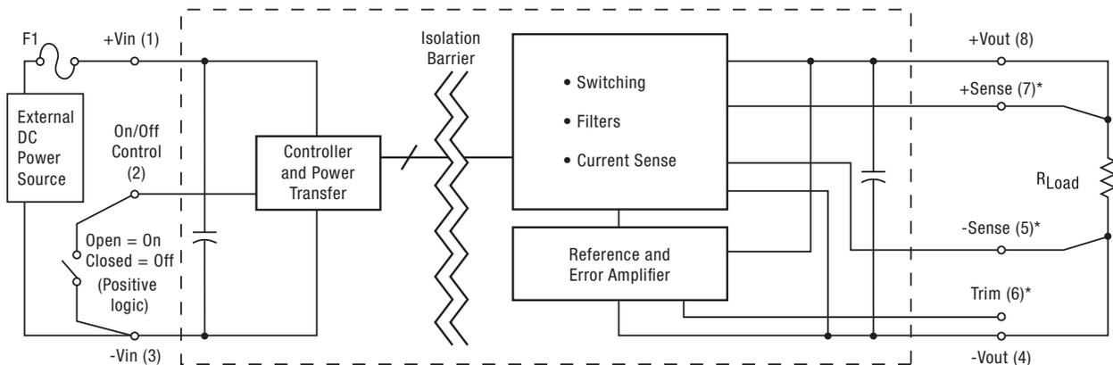
Figure 1. Connection Diagram
