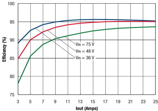
Efficiency vs. Output Current @ -40°C
