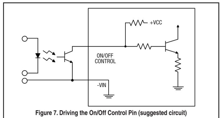
Figure 7. Driving the On/Off Control Pin (suggested circuit)
