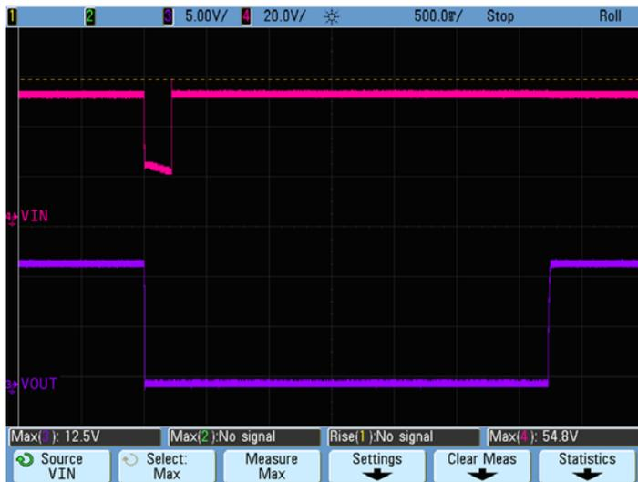
Scenario II: Vin recovers after more than 2.5s (restart delay time less than 15ms)
