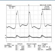
Figure 1. Vouts Output Ripple Top: No external capacitors
