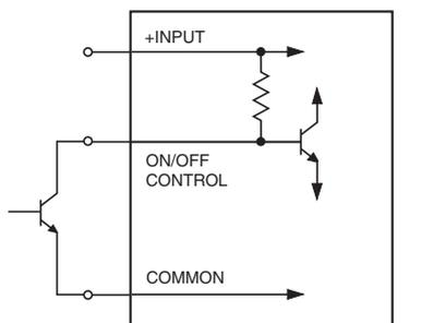
ON/OFF pin open: Logic High = DC/DC converter On
