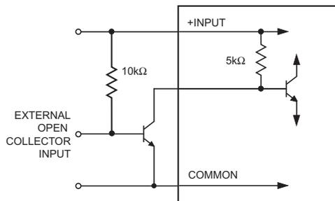
External Input Open: On/Off pin Low = DC/DC converter Off
