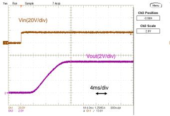
Fig.12-2-1. Start-up Waveform (Io=0A)
