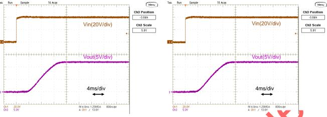
Fig.12-2-31. Start-up Waveform (Io=0A)
