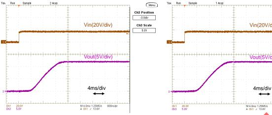
Fig.12-2-19. Start-up Waveform (Io=0A)
