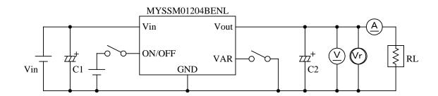
C1: Conductive Polymer Aluminum Solid Electrolytic Capacitor 100µF/50V
