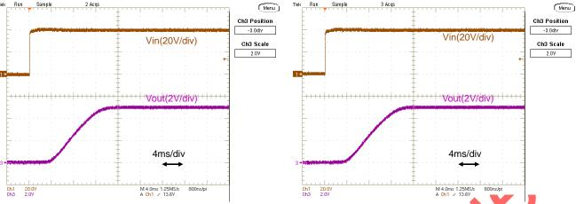
Fig.12-2-13. Start-up Waveform (Io=0A)
