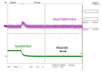
Fig.12-2-24. Load Transient Response  $(lo=3.5A\rightarrow 0)$
