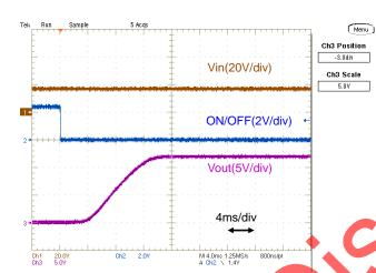
Fig.12-2-21. Start-up Waveform (Io=0A)
