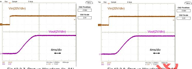
Fig.12-2-7. Start-up Waveform (Io=0A)
