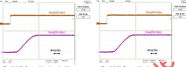
Fig.12-2-25. Start-up Waveform (Io=0A)
