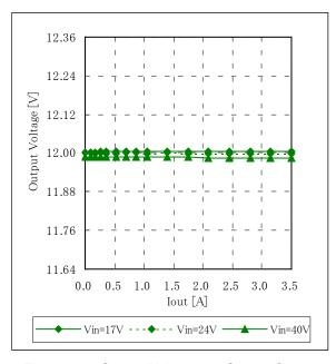
Fig.12-1-4. Output Voltage vs. Output Current
