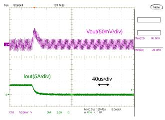
Fig.12-2-5. Load Transient Response (Io=  $0 \rightarrow 3.5A$ )
