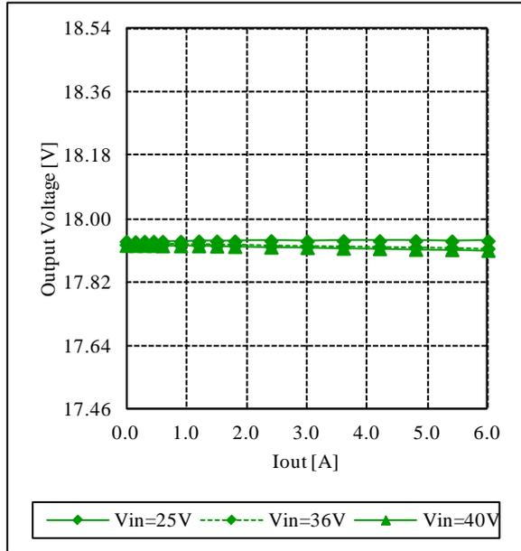
Fig.12-1-4. Output Voltage vs. Output Current
