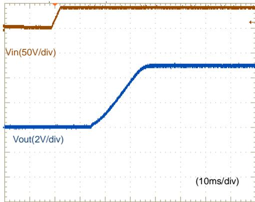
Fig.12-2-7. Start-up Waveform ( $I_o=0A$ )
