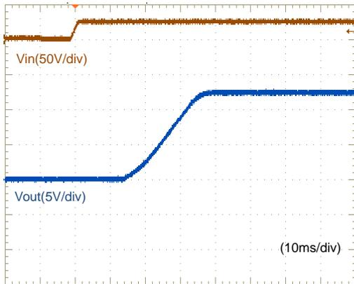
Fig.12-2-19. Start-up Waveform ( $I_o=0A$ )
