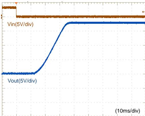
Fig.12-2-15. Start-up Waveform ( $I_o=0A$ )
