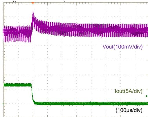
Fig.12-2-18. Load Transient Response
