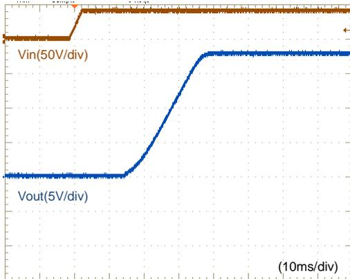
Fig.12-2-13. Start-up Waveform ( $I_o=0A$ )
