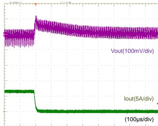
Fig.12-2-12. Load Transient Response
