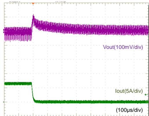
Fig.12-2-6. Load Transient Response
