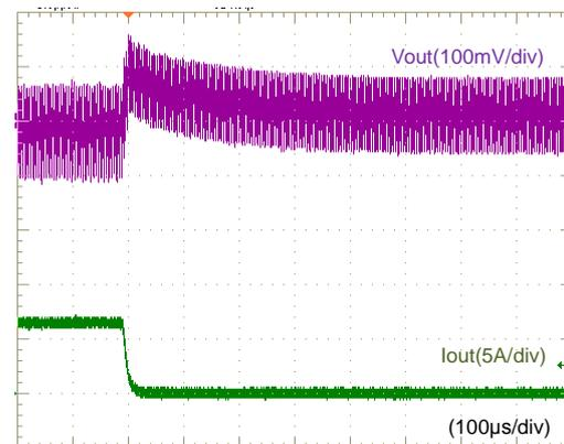
Fig.12-2-24. Load Transient Response
