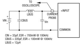
Figure 1. Measuring Input Ripple Current
