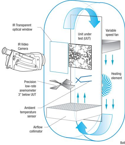
Figure 6. Vertical Wind Tunnel
