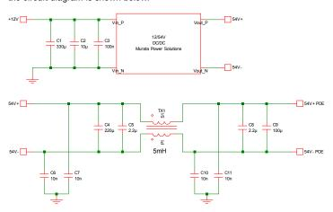
Figure 5. Conducted Emissions Test Circuit
