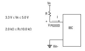
Figure 3. External circuit configuration for PGOOD signal
