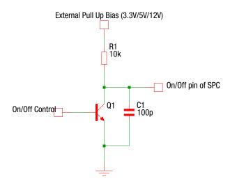
Figure 2. Remote On/Off Control Circuit
