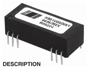
The HB01U Series offers a wide selection of input and output voltages to choose from. Each model is offered in a 24-pin DIP or SMD package and has an input to output isolation rating of 2500Vrms making it ideal for applications requiring high isolation. The dielectric withstand characteristics of each converter are measured in production to ensure barrier integrity.
