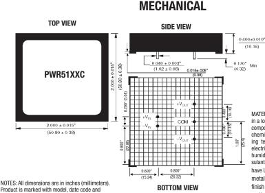
MATERIAL: Units are encansulated in a low thermal resistance molding compound that has excellent chemical resistance, wide operating temperature range, and good electrical properties under high humidity environments. The encapsulant and outer shell of the unit have UL94V-0 ratings. Lead base metal is phosphor bronze; lead finish is 100-300 micro-inches matte tin over a barrier layer of 5-40 micro-inches of nickel.
