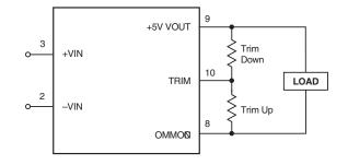
Figure 8. Trim Connections Using Fixed Resistors
