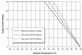
Figure 2a. Temperature Derating Without Heat Sink
