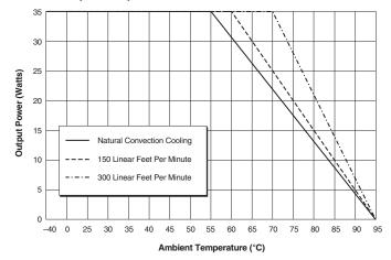
Figure 4a. Temperature Derating Without Heat Sink
