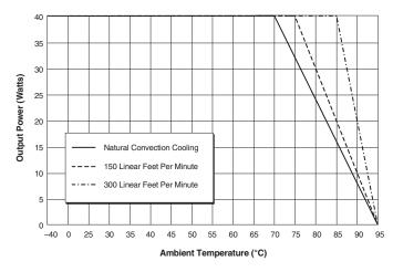
Figure 5a. Temperature Derating Without Heat Sink
