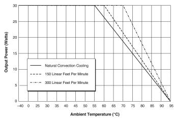
Figure 3a. Temperature Derating Without Heat Sink
