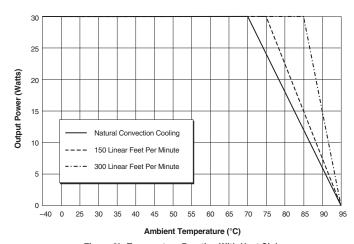
Figure 3b. Temperature Derating With Heat Sink
