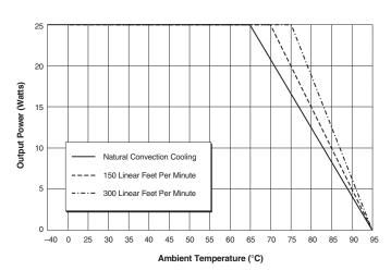
Figure 2b. Temperature Derating With Heat Sink
