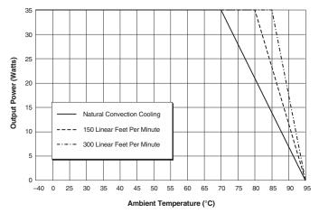
Figure 4b. Temperature Derating With Heat Sink
