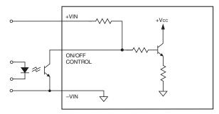
Figure 5. Driving the Negative Logic On/Off Control Pin
