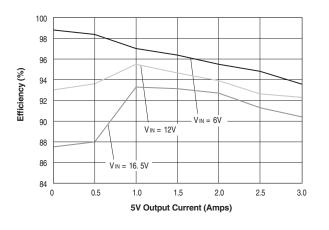
Efficiency vs. Output Current and Input Voltage (Model UNS-5/3)
