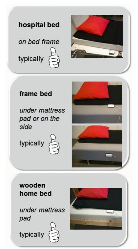
Figure 5. Examples of good SCA11H attachment positions
