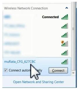
Figure 7. Example SCA11H's configuration network.
