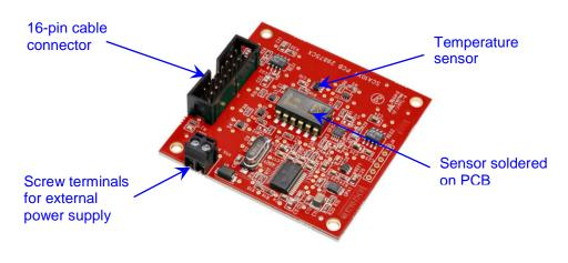
Figure 2. Extension board (SCA10xT PCB)
