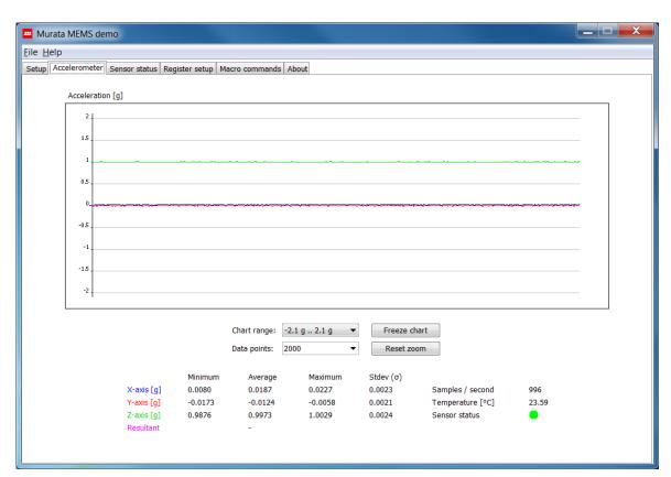
Figure 17. Output data view for accelerometer sensors
