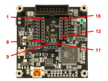
Figure 45. Chip carrier pin numbering
