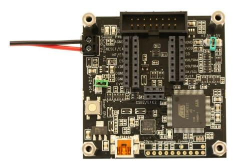
Figure 46. Evaluation board with external power cable inserted
