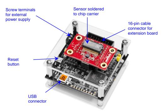
Figure 1. MEMS Evaluation Board
