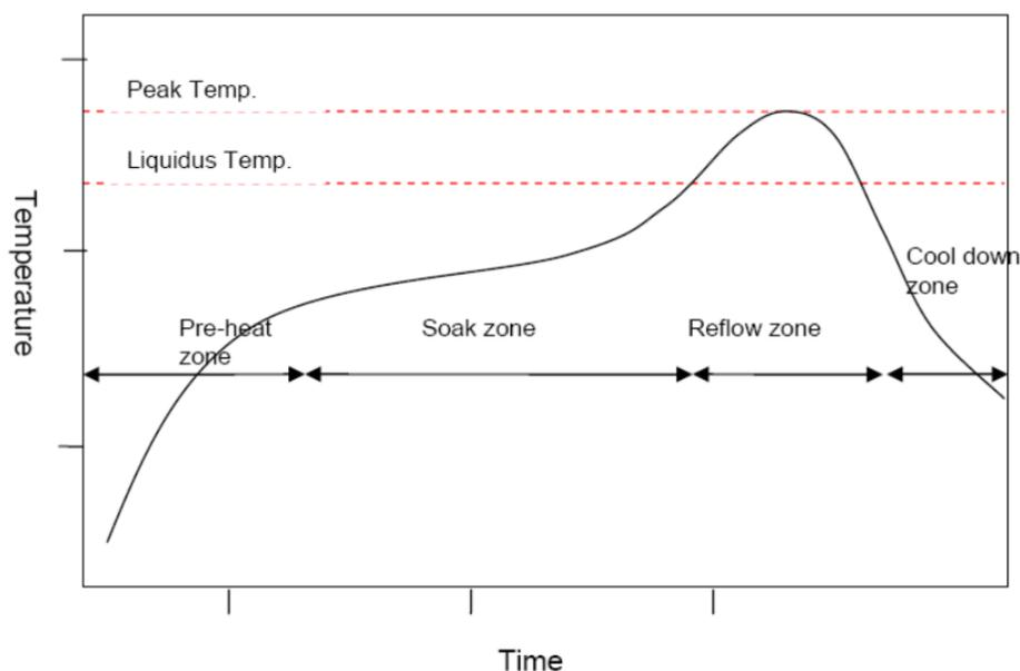
**Figure 7.** Typical convection reflow soldering phases and profile.
