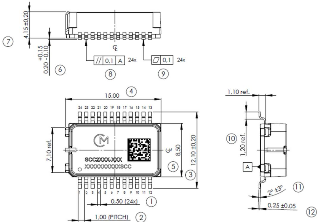
**Figure 2.** Outline and dimensions for DIL-24 package. Dimensions are in millimeters [mm]. All tolerances are according to ISO 2768-f unless otherwise specified.
