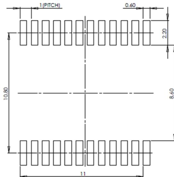
**Figure 6.** PCB pad lay-out for the DIL-24.
