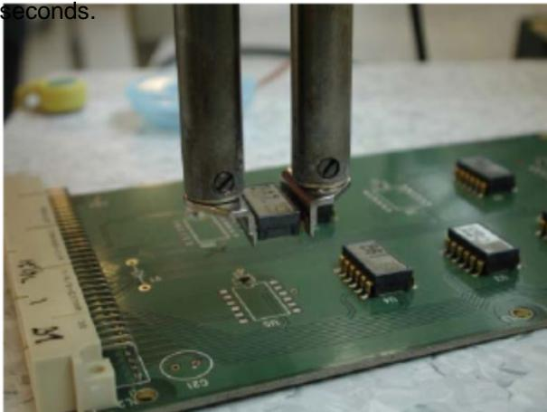
**Figure 13.** Immediately after solder melting, component is lifted.
