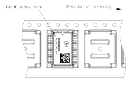
Figure 4. Package orientation on the tape and unreeling direction on tape.
