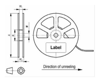
Figure 5. Reel dimensions. All dimensions are in millimeters [mm].
