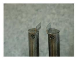
Figure 10. Thermal tweezers, Pace Thermotweez. Figure 11. Tool head, Pace 1121-0416-P1.
