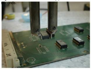
Figure 13. Immediately after solder melting, component is lifted.
