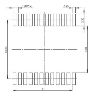
Figure 6. PCB pad lay-out for the DIL-24.
