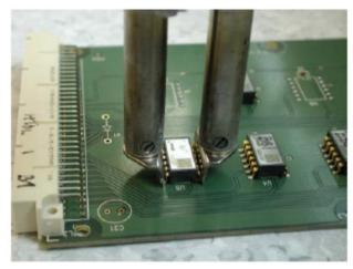
Figure 12. Tool head is carefully pressed around component and kept in this position for few
