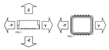
Figure 3. Accelerometer measuring directions
