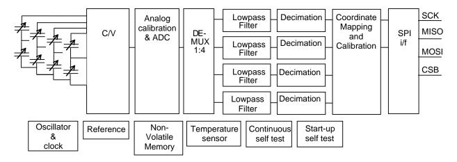
Figure 1. SCA2120-D06 Block diagram
