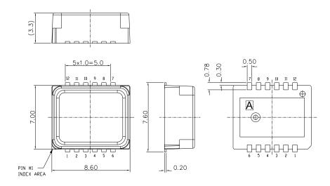
Figure 4. Housing dimensions
