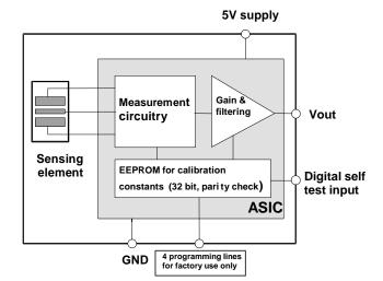
Figure 1. Functional block diagram.
