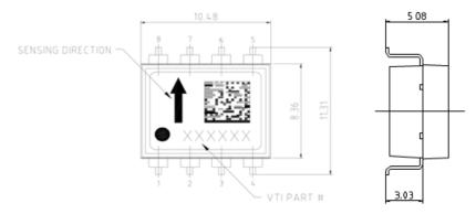
Figure 8. Mechanical dimensions (mm).
