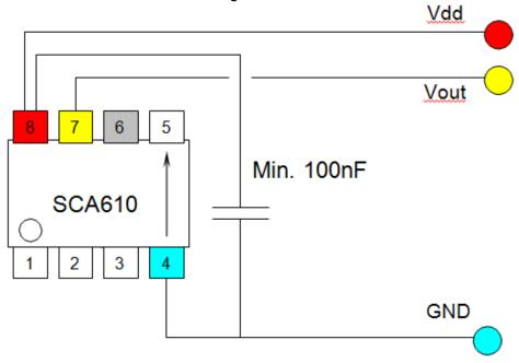
**Figure 3.** Electrical connection of SCA610 component.
