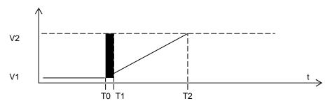
Figure 2. V<sub>DD</sub> Start-up sequence.
