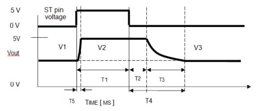
Figure 7. Self test wave forms.
