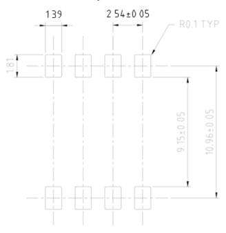
Figure 9. Recommended PCB layout (mm).
