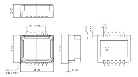
Figure 4. Housing dimensions
