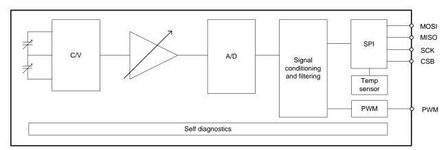
Figure 1. SCA830-D06 Block diagram
