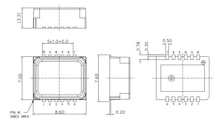
Figure 4. Housing dimensions
