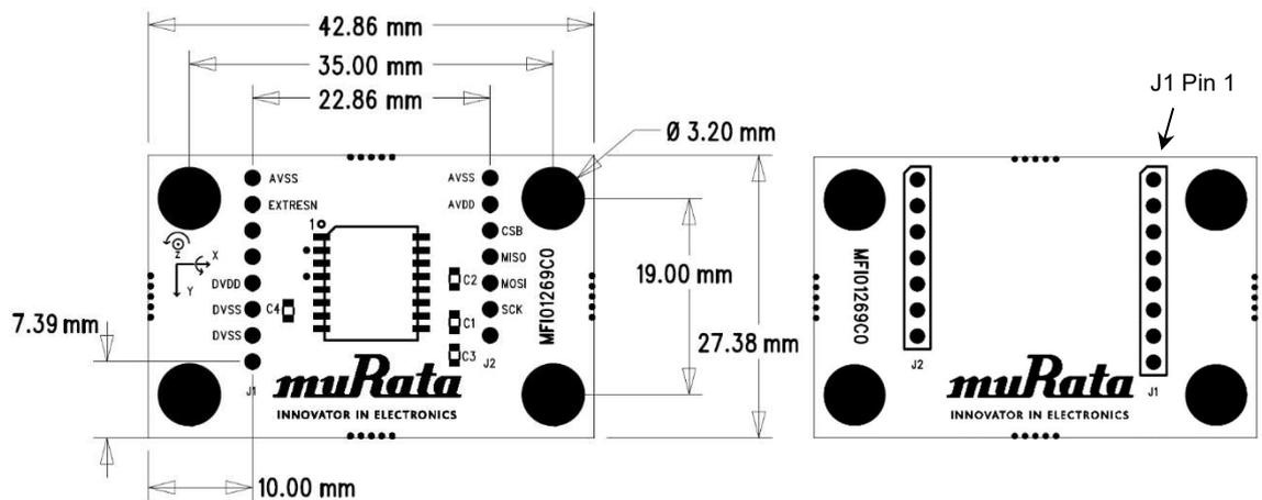
Figure 3. TOP (left) and BOTTOM (right) view assembly drawings for SCC400T PCB (aspect ratio not 1:1).
