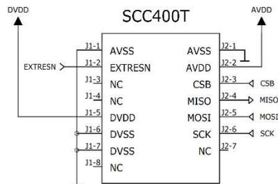
Figure 1. SCC400T PCB pinout and external connections.
