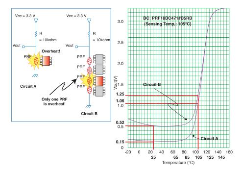
Fig. 3: Overheat sensing circuit for multiple locations using the Posistor PTC thermistor and its output voltage ( $V_{out}$ )
