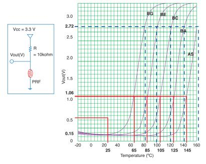
Fig. 2: Overheat sensing circuit using Posistor PTC thermistor and its output voltage  $(V_{\text{out}})$
