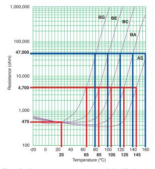
Fig. 1: Resistance temperature characteristic of Posistor PTC thermistor
