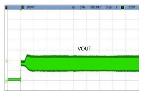
Typical sample at VBUS=5.0V, +25°C [VOUT] Vertical: 0.2V/div.,
