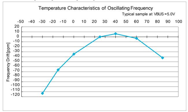
All above results have been measured using a RSL10 evaluation board, provided by On Semiconductor, with optimized circuit conditions for the WMRAG32K76CS1C00R0. Please refer to TCD-18-0165, issued by Murata, for more details.
