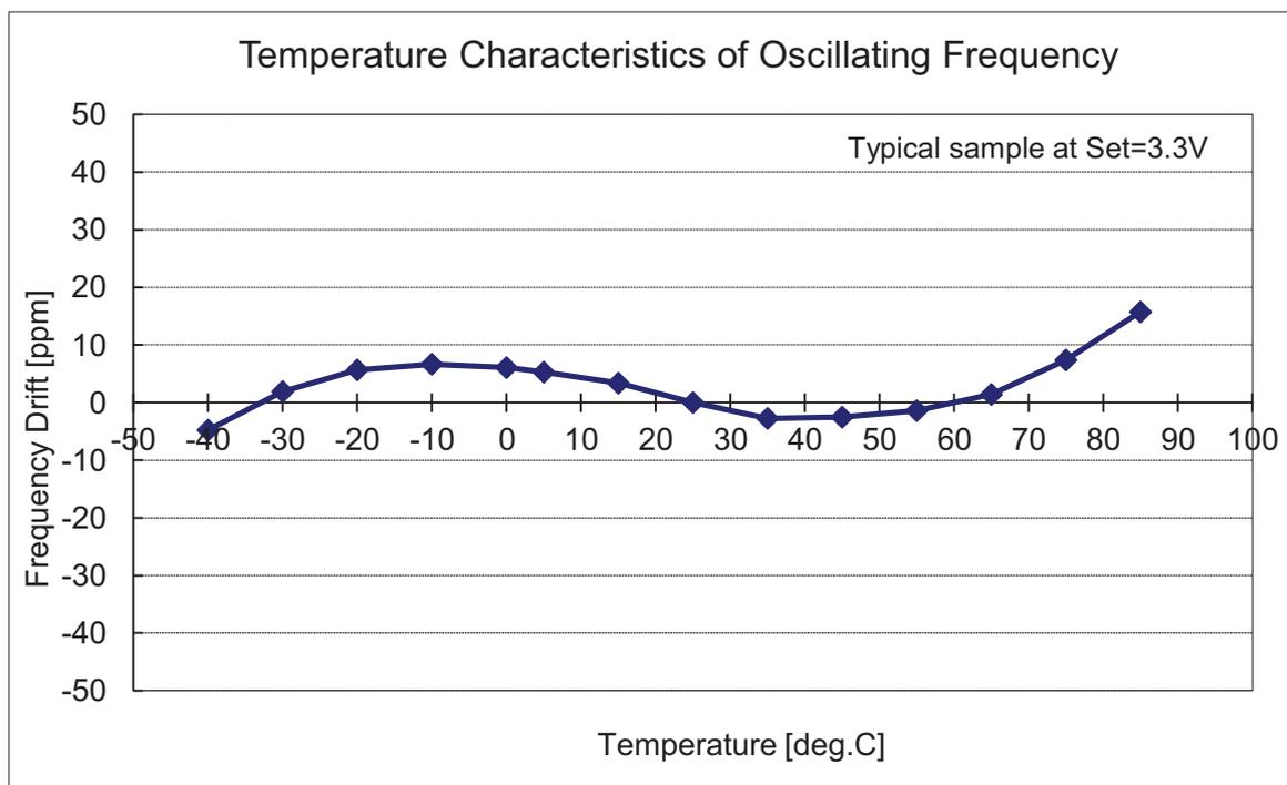
All of above results have been measured on evaluation board of nRF52xxx (PCA10040) from Nordic, with optimized circuit conditions for XRCGB32M000F2P10R0. Refer TCD-16-0017, issued by Murata, for more detail.
