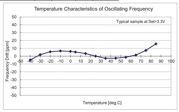
All of above results have been measured on evaluation board of nRF52xxx (PCA10040) from Nordic, with optimized circuit conditions for XRCGB32M000F2P10R0. Refer TCD-16-0017, issued by Murata, for more detail.
