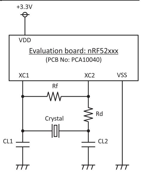
Figure of oscillation circuit
