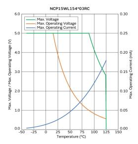
Max. Voltage, Max. Operating Voltage/Current **Reduction Curve**
