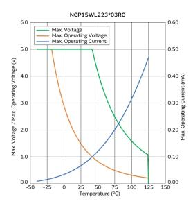
Max. Voltage, Max. Operating Voltage/Current Reduction Curve
