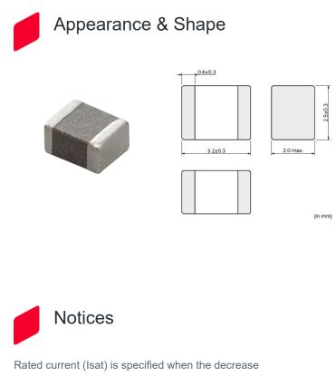
Rated current (Isat) is specified when the decrease of the initial inductance value at 30%. Rated current (Itemp) is specified when temperature of the inductor is raised 40°C by DC current.
